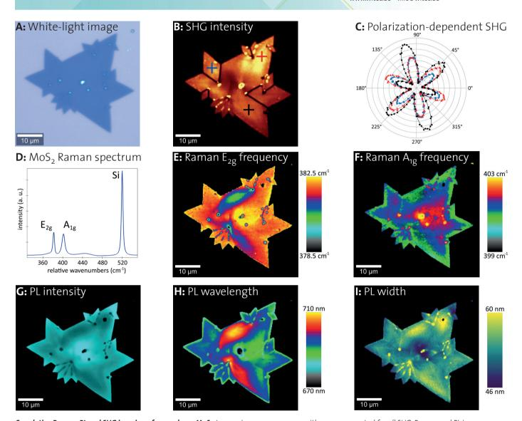
Correlative Raman, PL and SHG imaging of mono-layer MoS<sub>2</sub>. Image size:  $50 \mu m \times 50 \mu m$  with 200 nm per pixel for all SHG, Raman and PL images.
