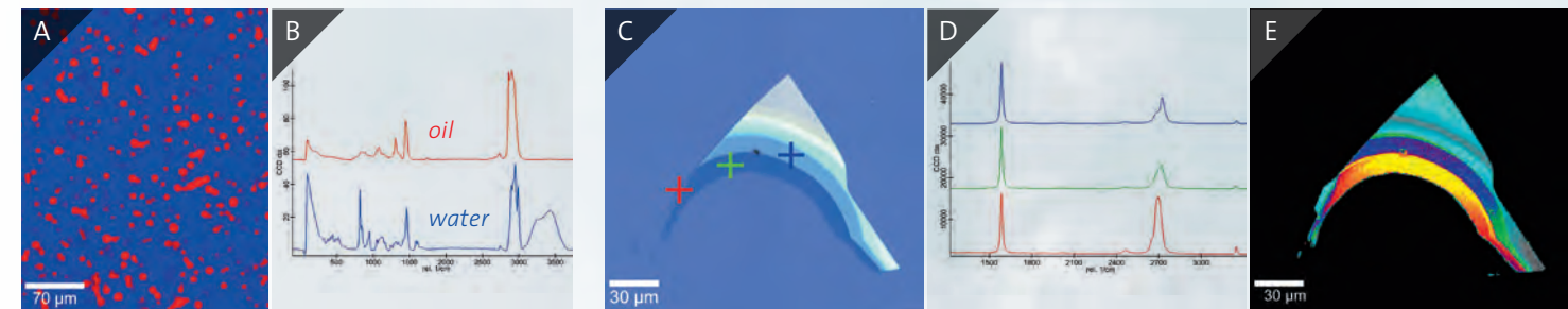
Large-area Raman map (A) of a pharmaceutical pain relief ointment (emulsion) and corresponding spectra of oil and water with the dissolved active ingredient (B).
